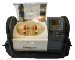
System for diagnosis and analyze of isolation MIDAS micro 2883
